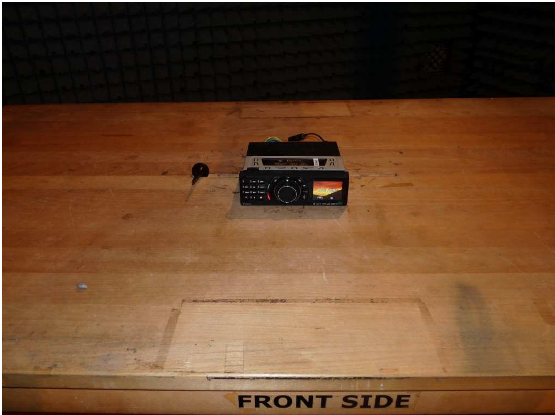
Photo 2: Test setup for radiated measurements (Enclosure, 30 MHz to 1 GHz)
