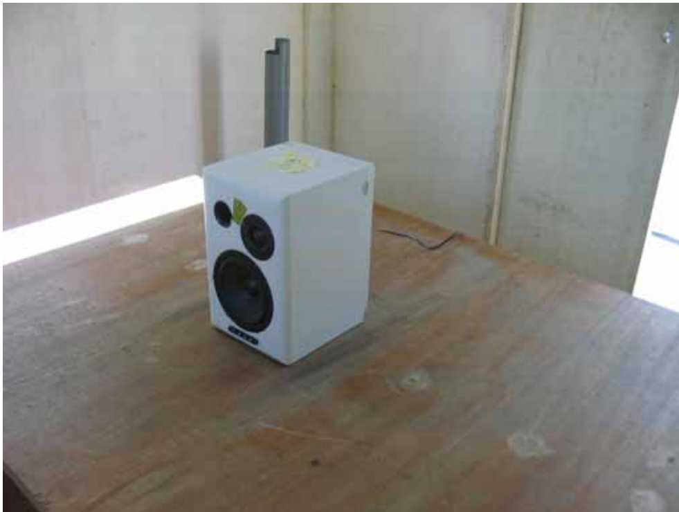
Open area test site, test set up of the radiated measurement (front view)
