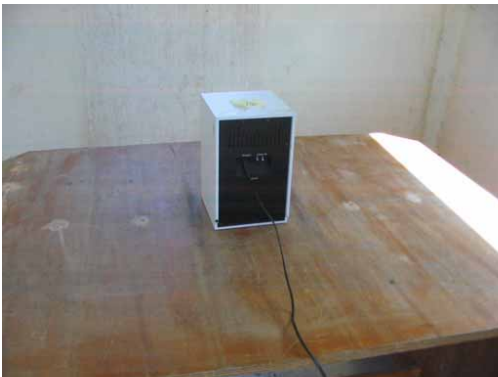
Open area test site, test set up of the radiated measurement (rear view)
