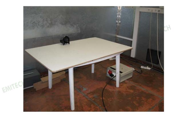
TEST SET UP RADIATED MEASUREMENT
