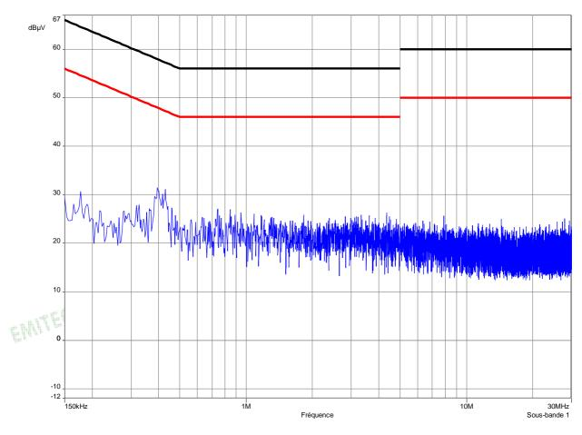
RBW filter: 10 kHz VBW filter: 30 kHz
