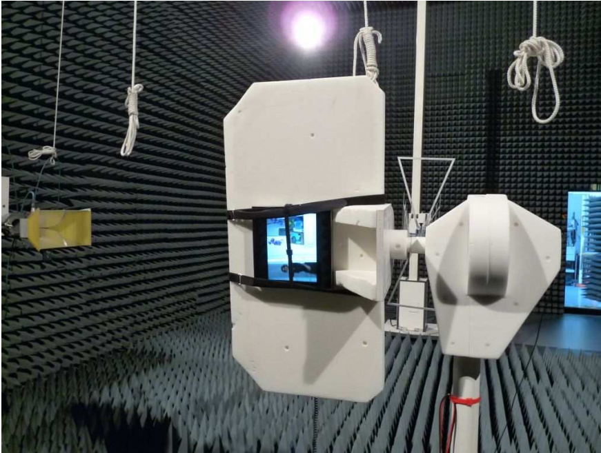
Photo 1: Test setup for radiated measurements
