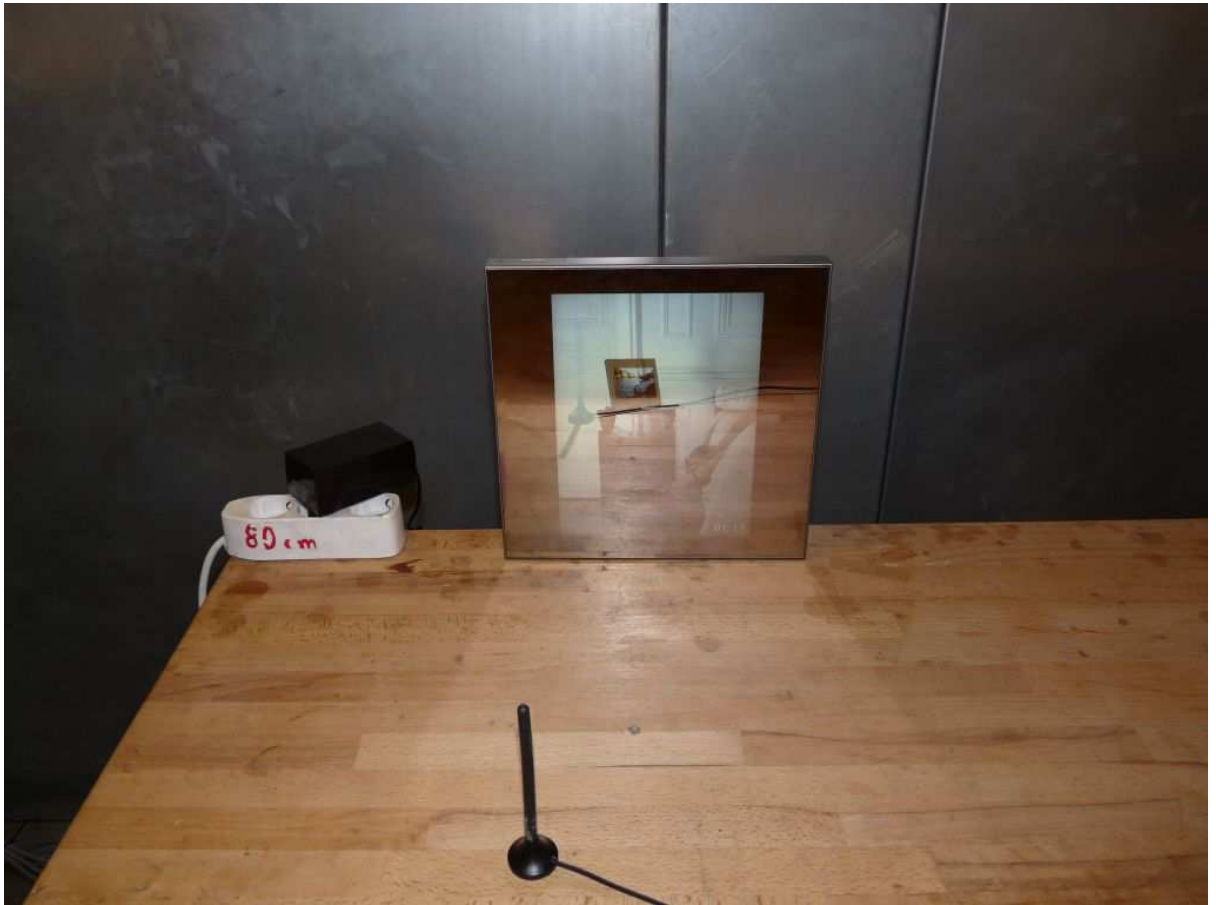
setup for the test AC conducted emissions
