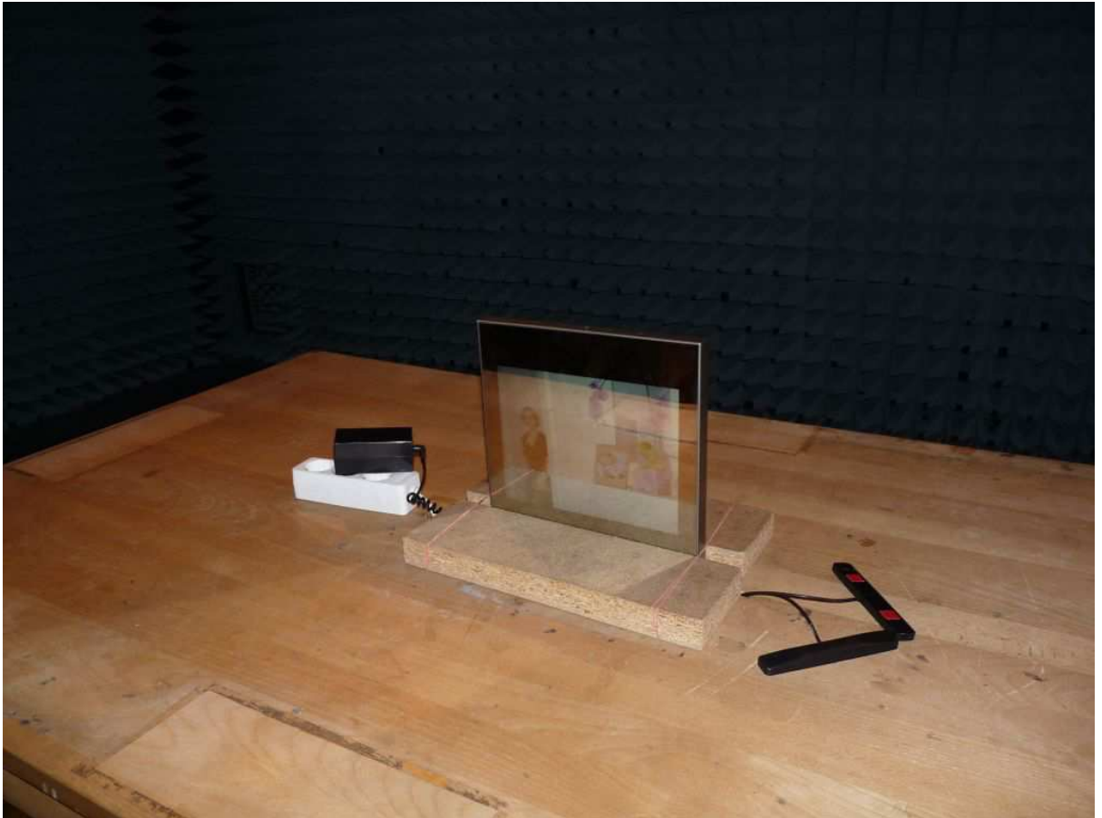
setup for the test radiated emissions
