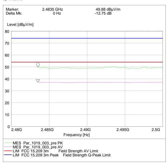
Radiated measurement (higher band edge)
