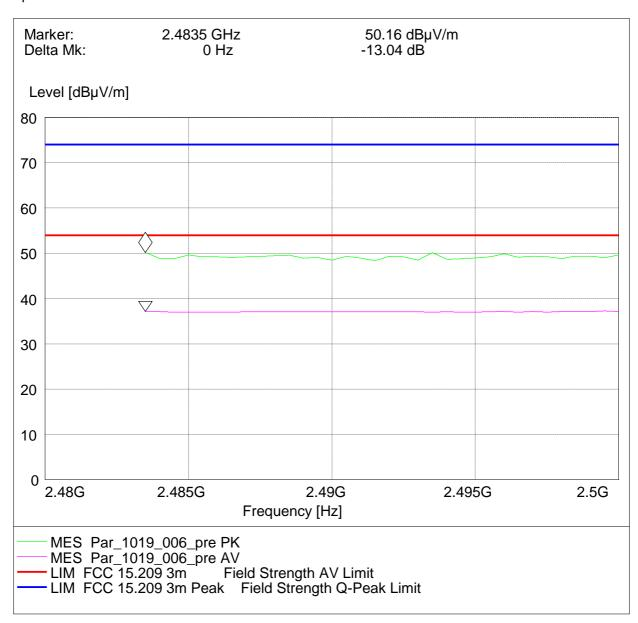
Radiated measurement (higher band edge)
