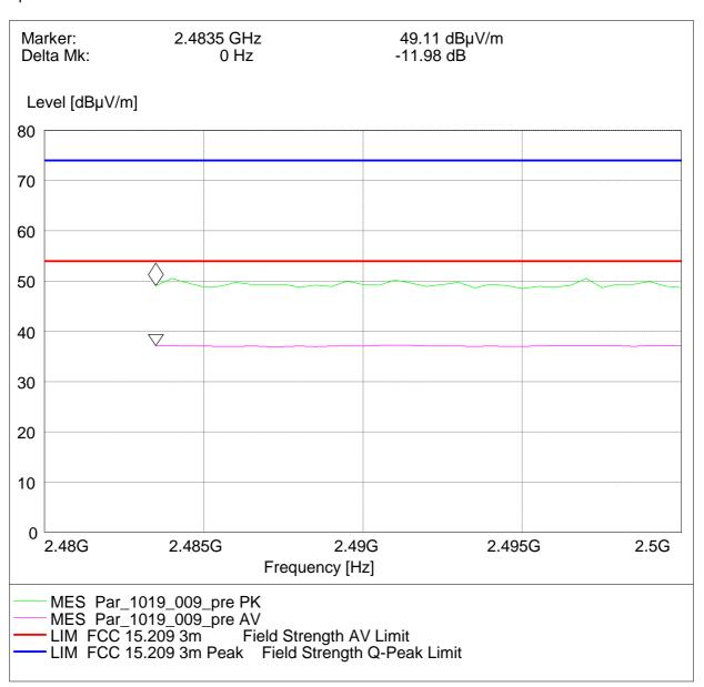
Radiated measurement (higher band edge)
