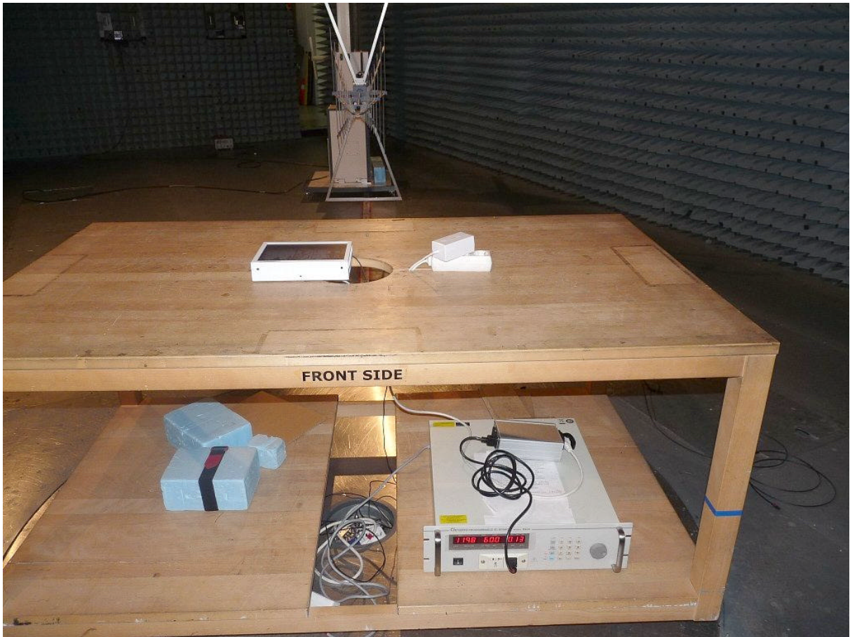
Photo 2: Test setup for radiated measurements (Enclosure, 30 MHz to 1 GHz) (besides for op-mode "colo" and tests for unintentional transmission)
