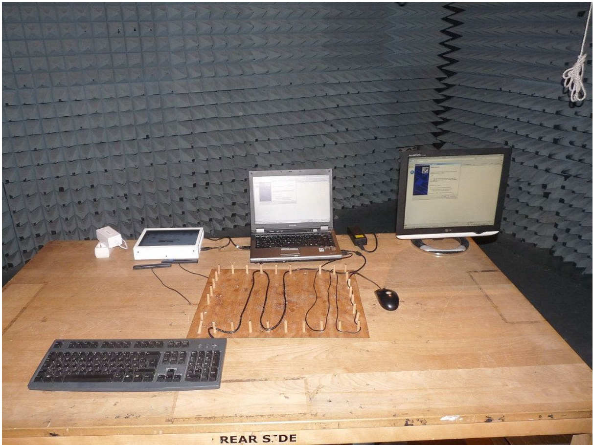
Photo 3: Test setup for radiated measurements (Enclosure, 30 MHz to 1 GHz) (for op-mode "colo" and tests for unintentional transmission)
