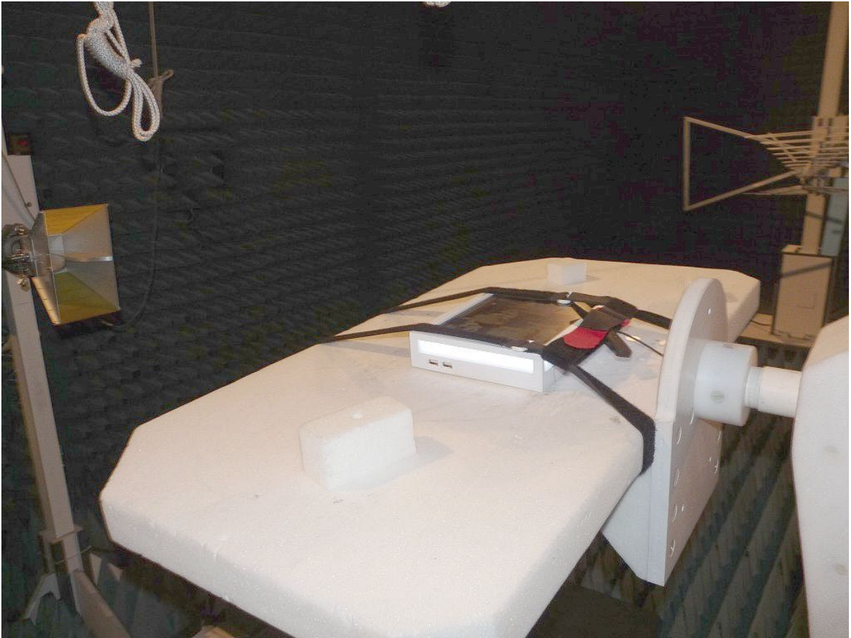
Photo 4: Test setup for radiated measurements (Enclosure, above 1 GHz)
