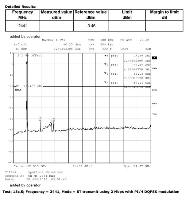
Result:PassedSetup No.:A03Date of Test:2012/07/10 15:21Body:FCC47CFRChIPART15c247RADIO FREQUENCY DEVICESTest Specification:FCC part 2 and 15
