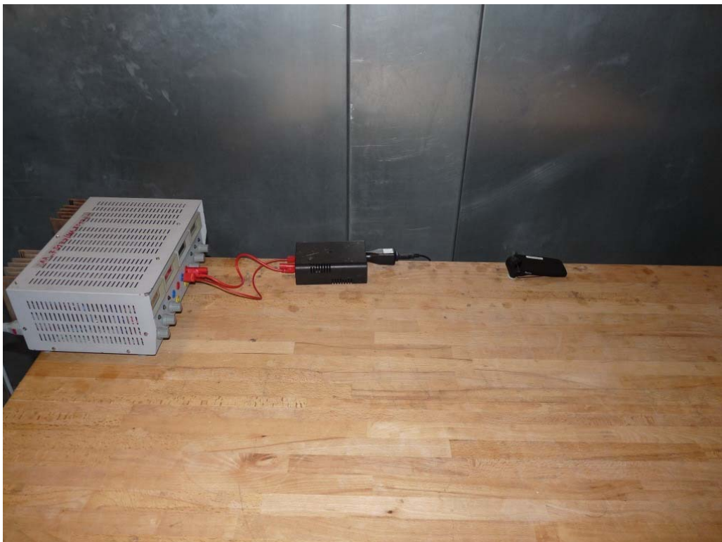
Photo 6: Test setup for conducted measurements (DC Port)
