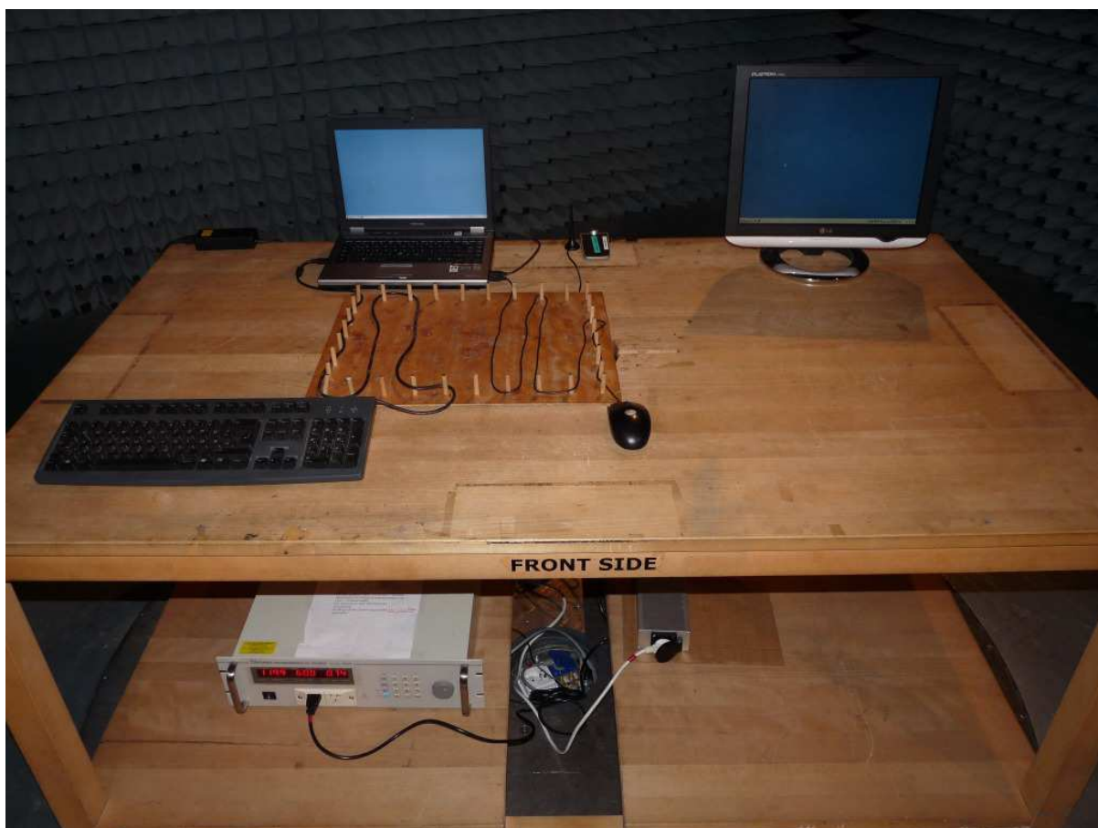
Test Setup Photo: radiated emissions (Computer peripheral Setup)
