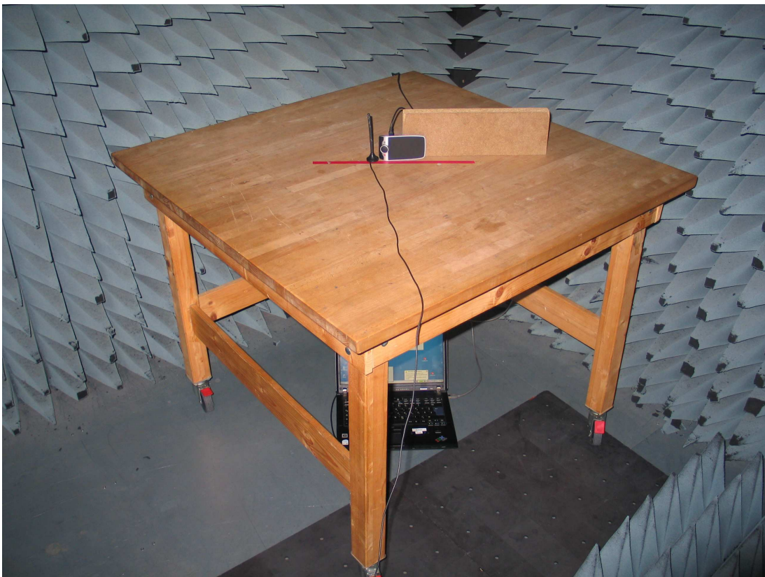
Photo 3: Test setup (Setup_a03) for radiated measurements (Enclosure, below 30 MHz)
