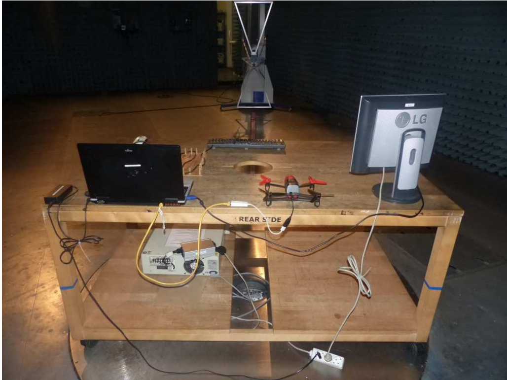
Photo 6: Test setup for radiated measurements (computer peripheral setup, EUT supplied by external DC power to enable USB data transfer to computer, unintentional radiator §15)
