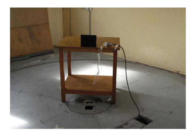
Antenna in front of the equipment when the turntable is at  $0^{\circ}\,$
