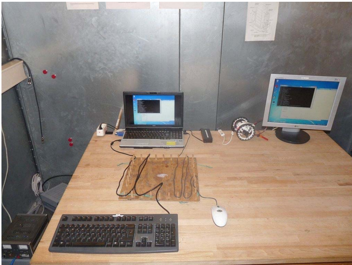
Photo 7: Test setup for conducted measurements (computer peripheral setup, EUT supplied by external DC power to enable USB data transfer to computer, unintentional radiator §15)
