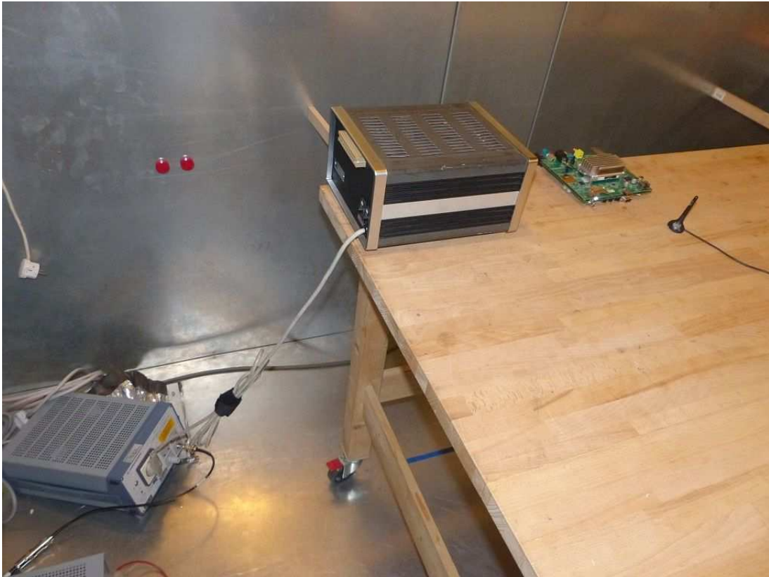
Photo 5: Test setup for conducted measurements (unintentional radiator §15)
