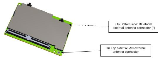
(\*) This connector exists also on internal BT antenna version of the module, but only for manufacturing purpose.
