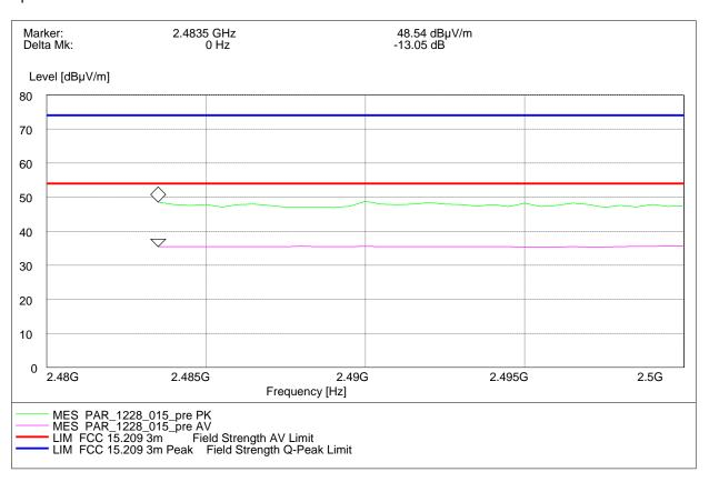
Radiated measurement (higher band edge)
