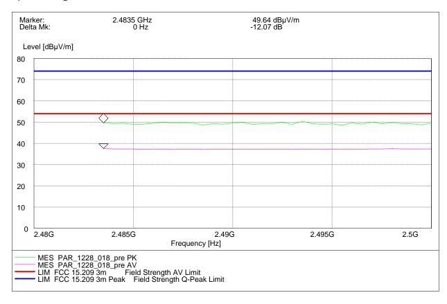
Radiated measurement (higher band edge)
