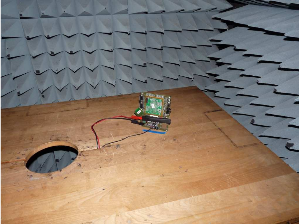
Photo 1: Test setup for radiated measurements (below 30 MHz)
