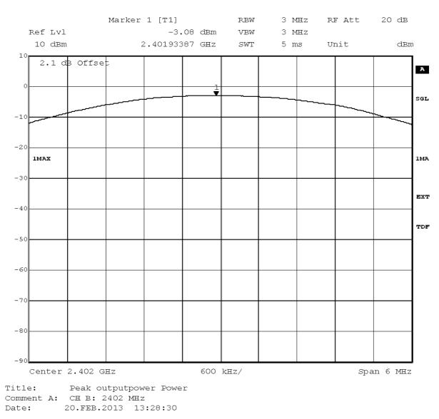
Test: 15c.4; Frequency = 2441, Mode = BT transmit using 1 Mbps with GFSK modulation
