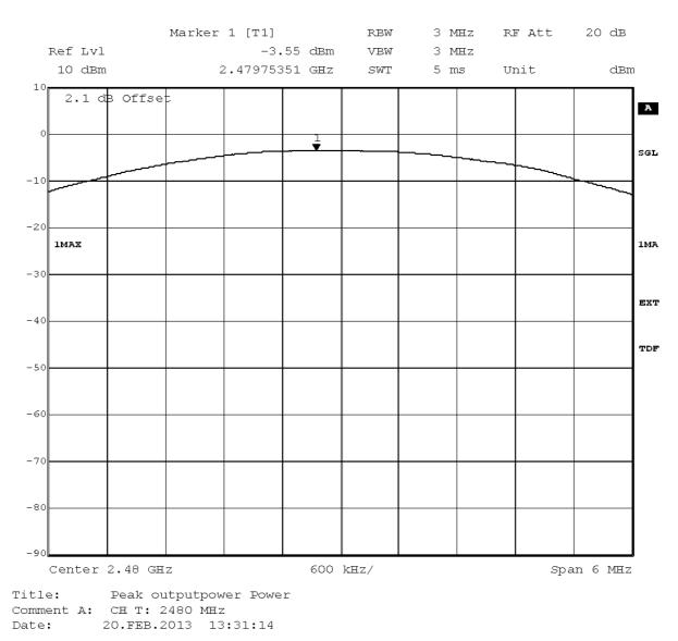
Test: 15c.4; Frequency = 2480, Mode = BT transmit using 2 Mbps with PI/4 DQPSK modulation
