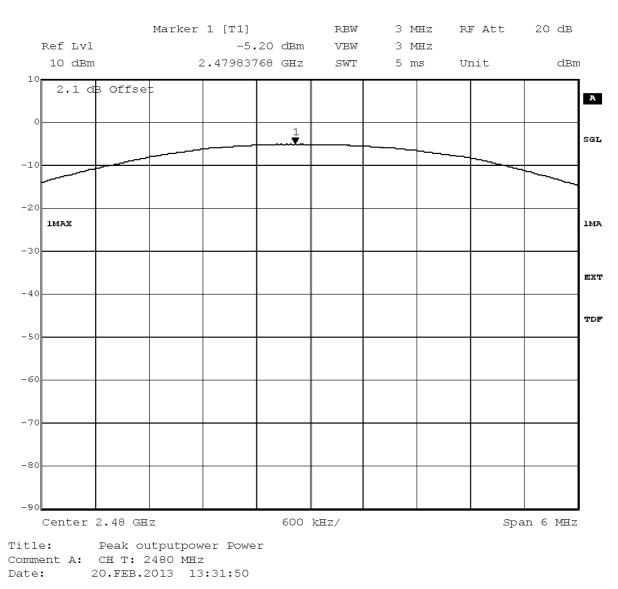
Test: 15c.4; Frequency = 2480, Mode = BT transmit using 3 Mbps with 8DPSK modulation
