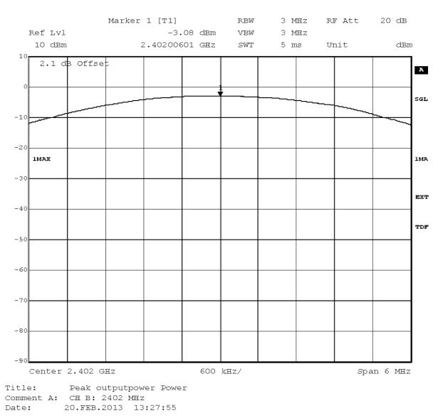
Test: 15c.4; Frequency = 2402, Mode = BT transmit using 3 Mbps with 8DPSK modulation
