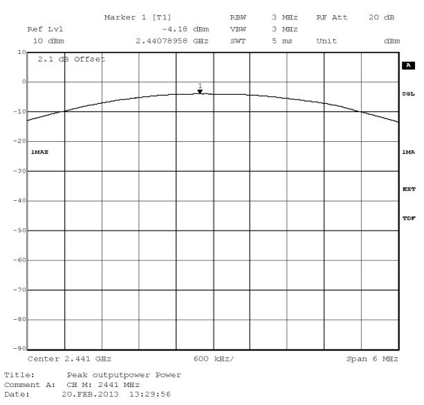
Test: 15c.4; Frequency = 2441, Mode = BT transmit using 3 Mbps with 8DPSK modulation
