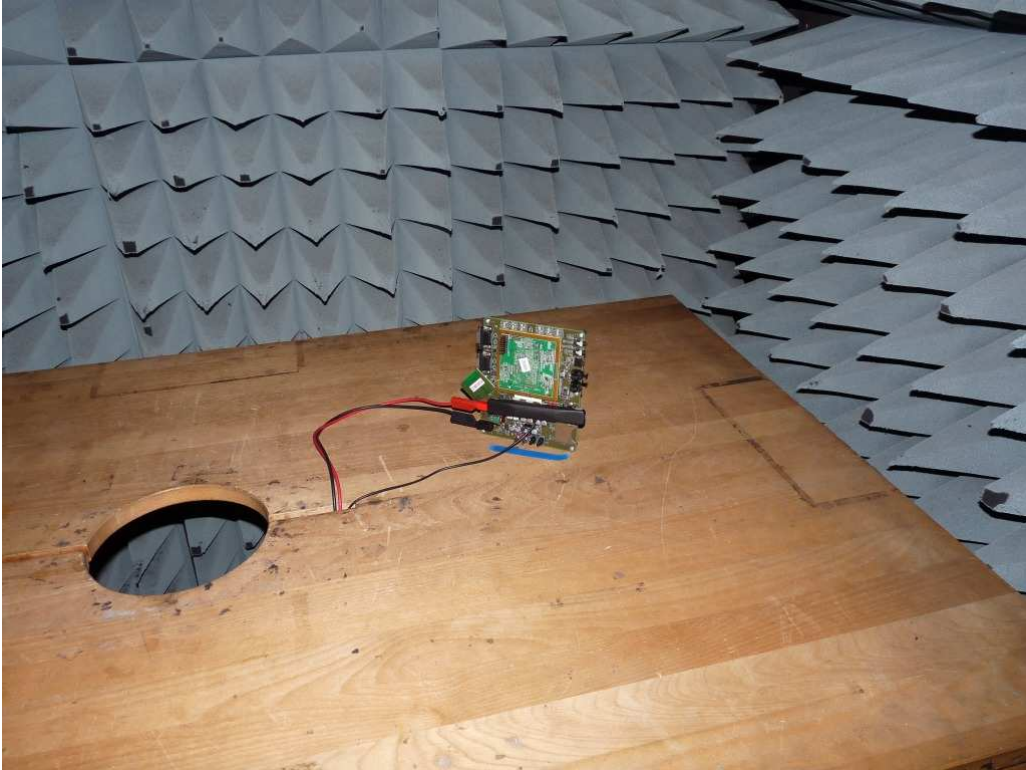
Photo 1: Test setup for radiated measurements (below 30 MHz)
