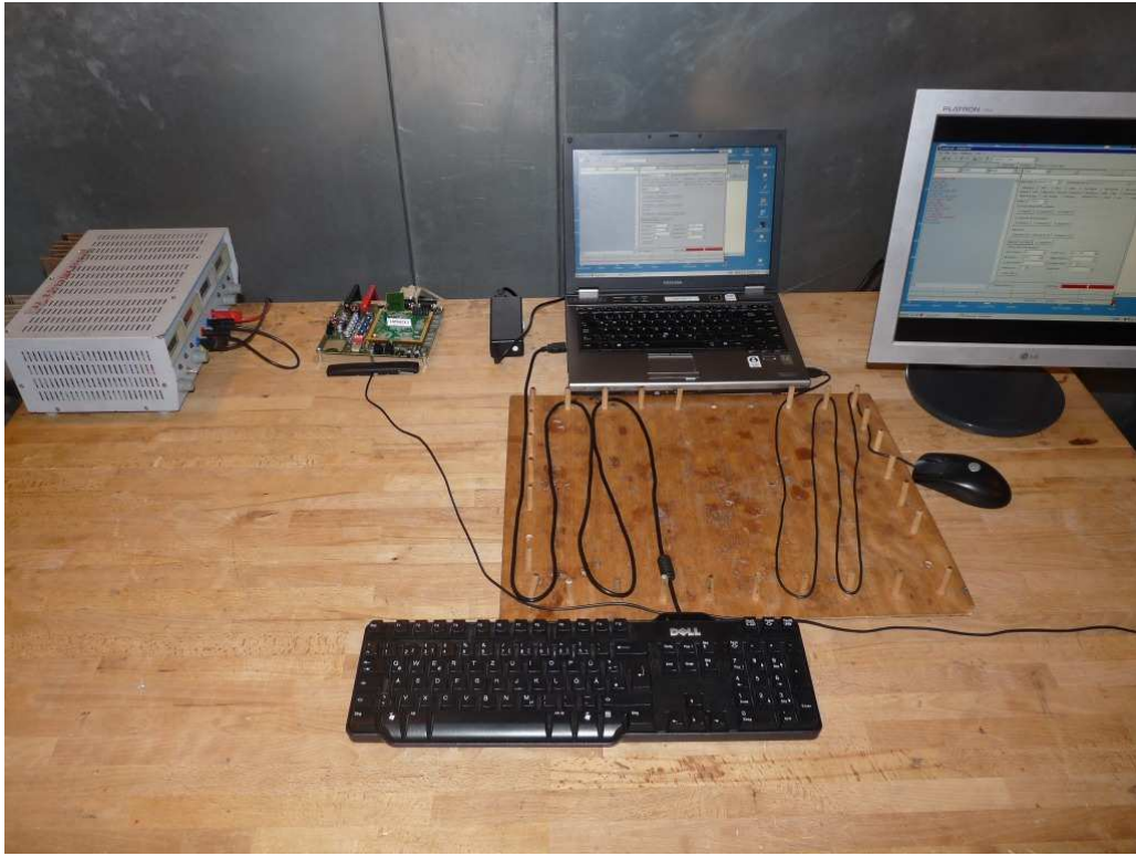
Photo 4: Test setup for conducted measurements, AC Mains
