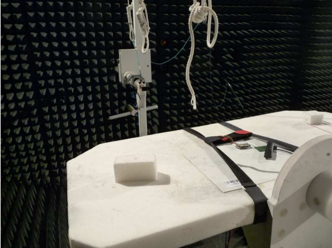
Photo 2: Test setup for radiated measurements (above 1 GHz)
