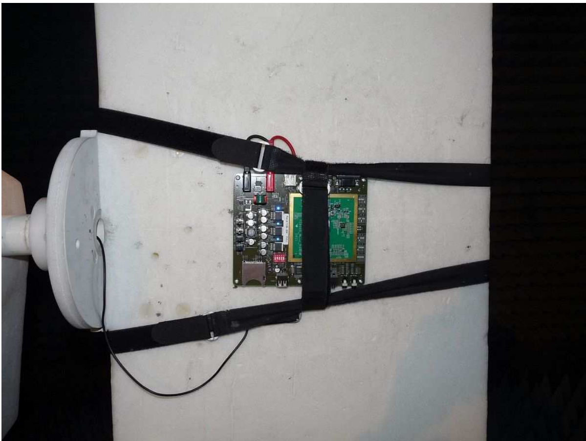
Photo 4: Test setup for radiated measurements (Enclosure, above 1 GHz) (EUT is fastened at the tilt device)a
