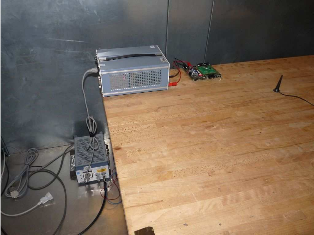
Photo 5: Test setup for conducted measurements (AC Port (power line))
