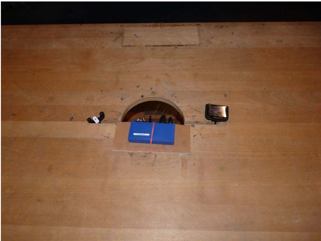
Photo 4: Setup_c01. Test setup for radiated measurements (Enclosure, 30MHz to 1GHz)
