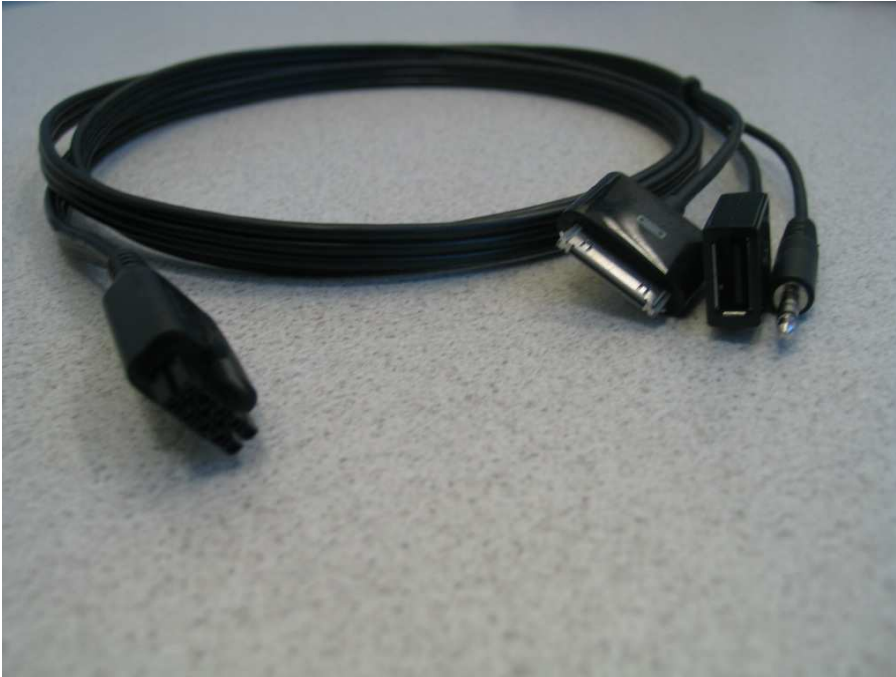
Photo 5: Ancillary Equipment (audio connection cable)
