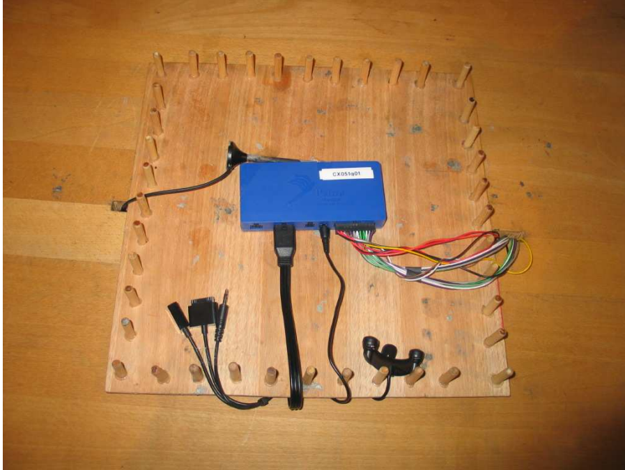
Photo 1: Test setup for radiated measurements
