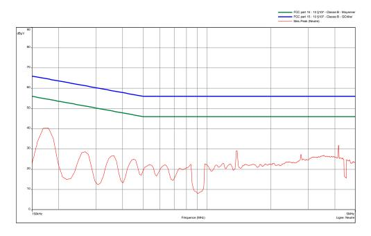
Curve N° 8: average measurement on the Line, for the frequency range: 150 kHz – 5 MHz
