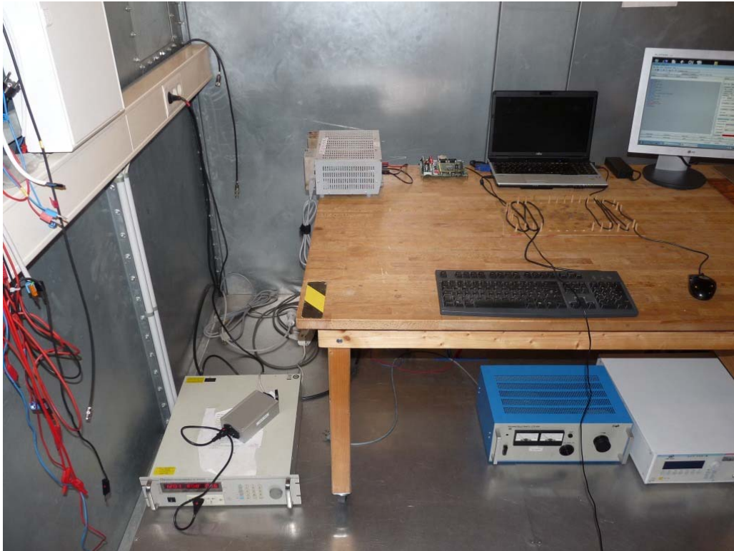
Photo 4: Test setup for conducted emissions measurements (150 KHz to 30 MHz), FCC 15.247 Module with external Antenna
