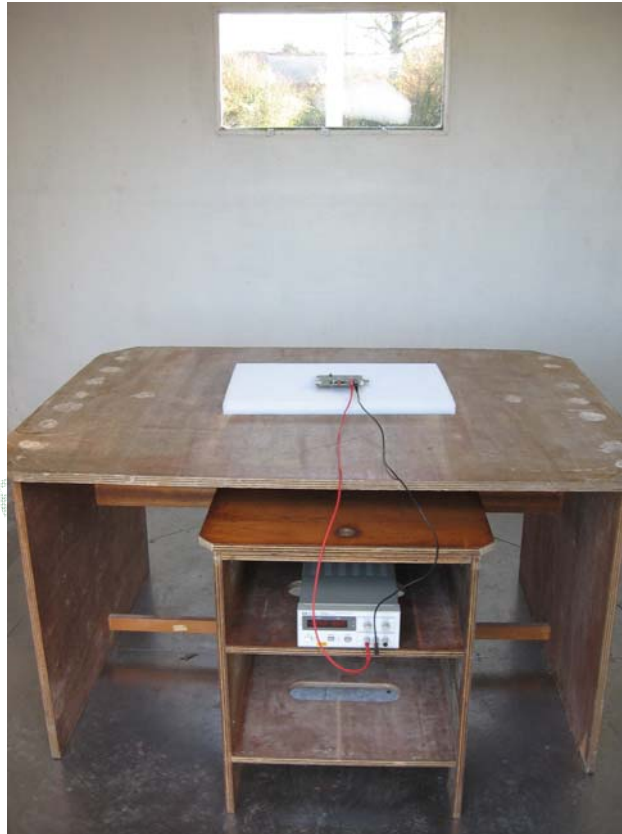
TEST SET UP FOR RADIATED MEASUREMENT
