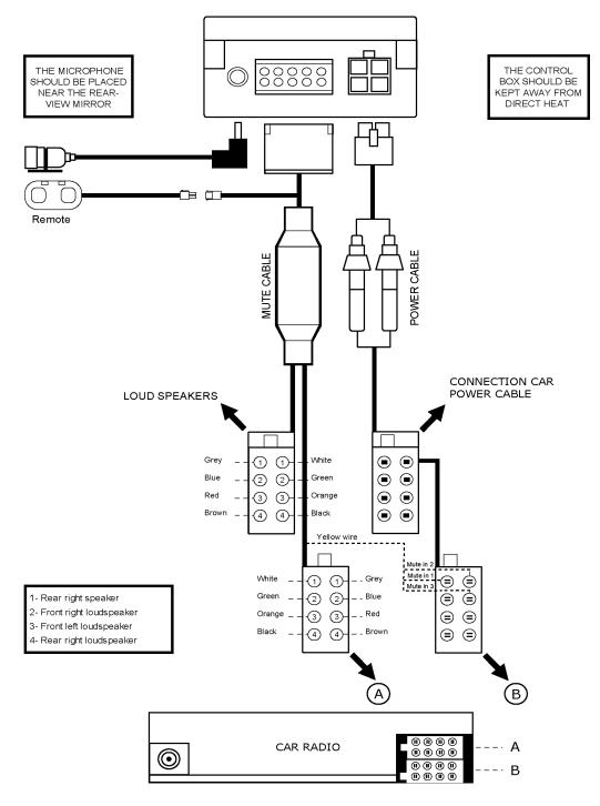
IMPORTANT: CK3000 operates only when ignition is switched on. Both lights on a Keypad must be on.
