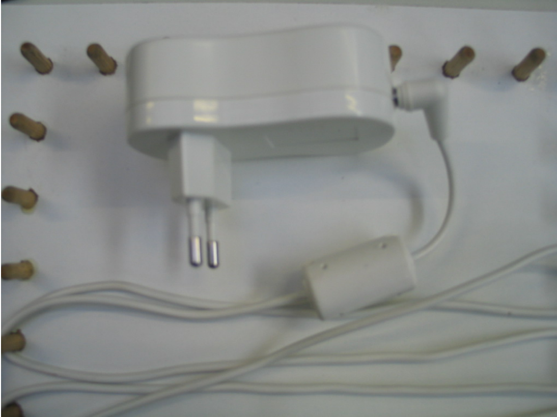
Photo 8: AC/DC power supply
