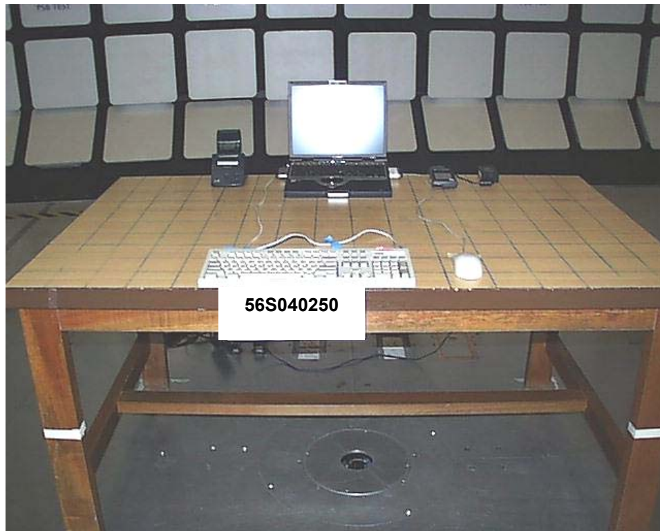
Radiated Emissions Setup (Front View)
