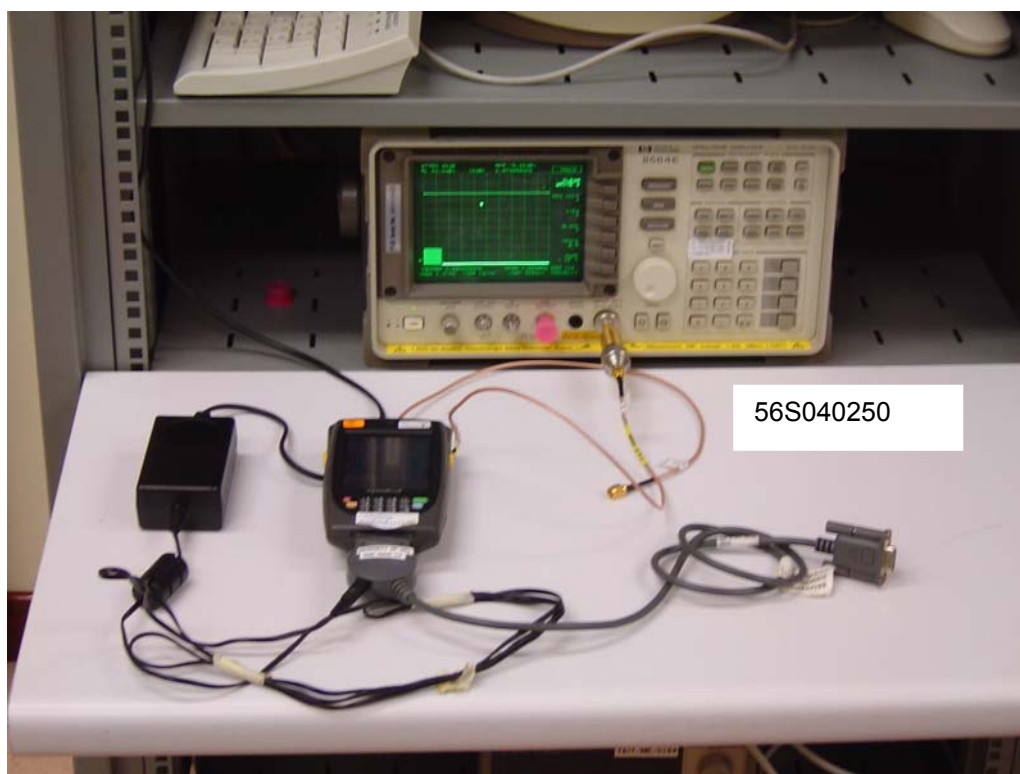
Peak Power Spectral Density Measurement Test Setup
