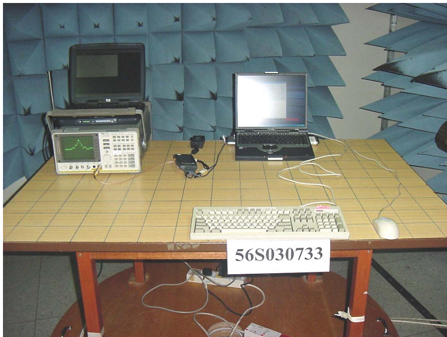
Average Frequency Dwell Time Measurement Test Setup
