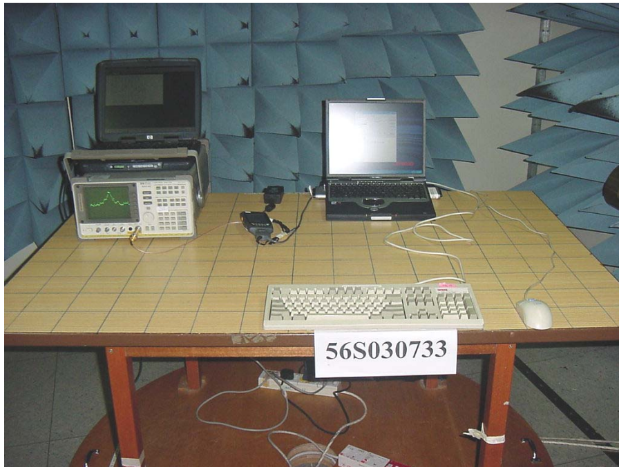
Carrier Frequency Separation Measurement Test Setup
