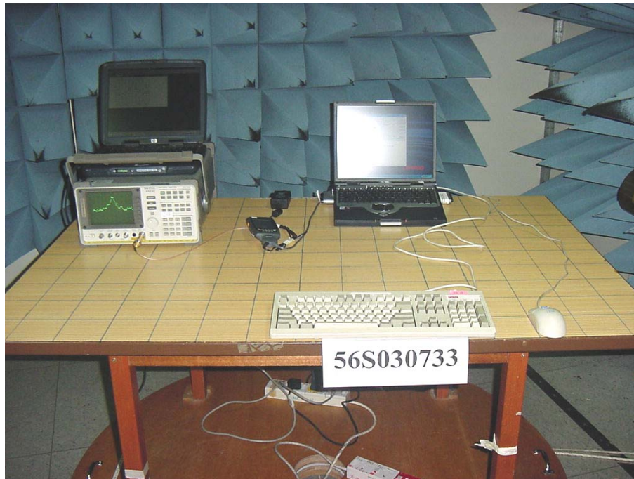
Number of Hopping Frequencies Measurement Test Setup
