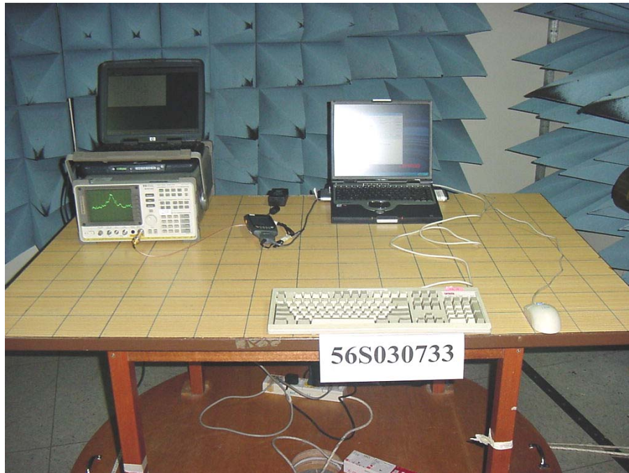
Spectrum Bandwidth Measurement Test Setup
