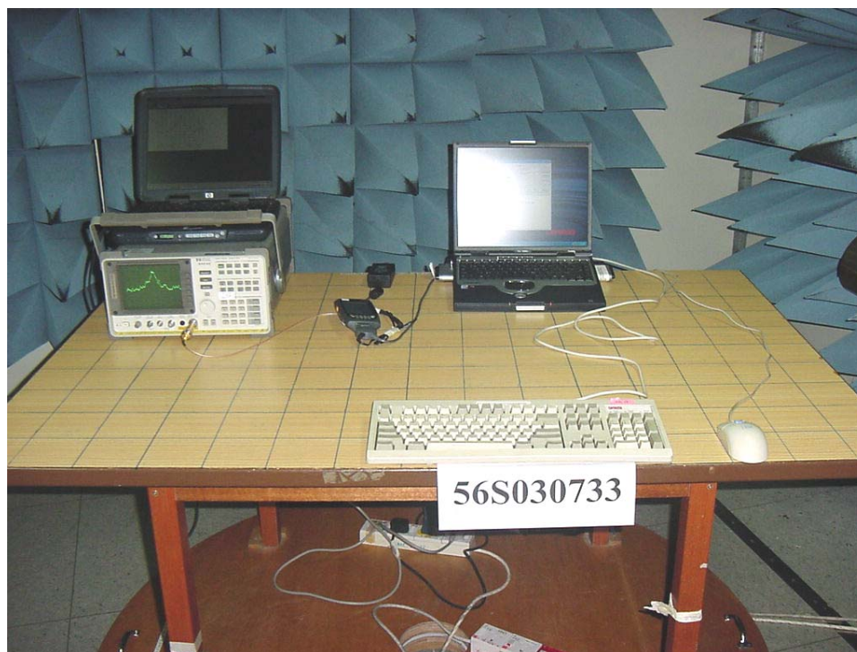
Average Frequency Dwell Time Measurement Test Setup
