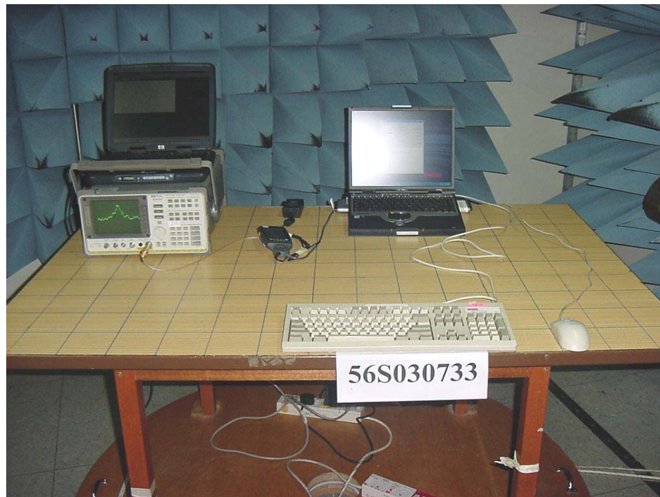
Carrier Frequency Separation Measurement Test Setup
