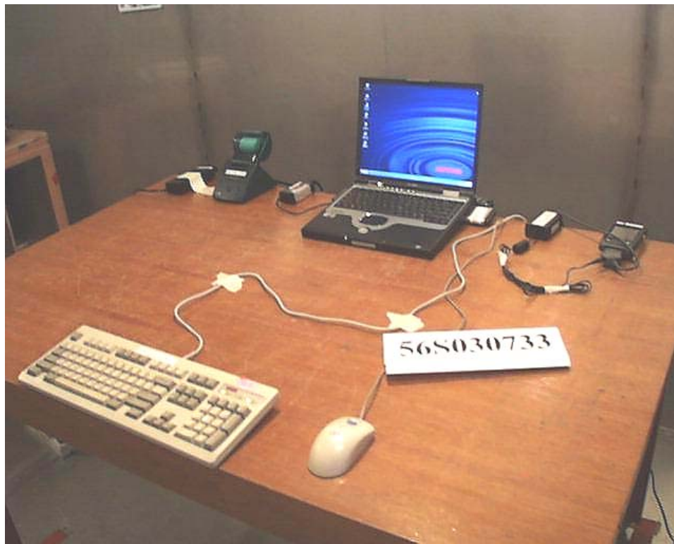
Conducted Emissions Setup (Front View)
