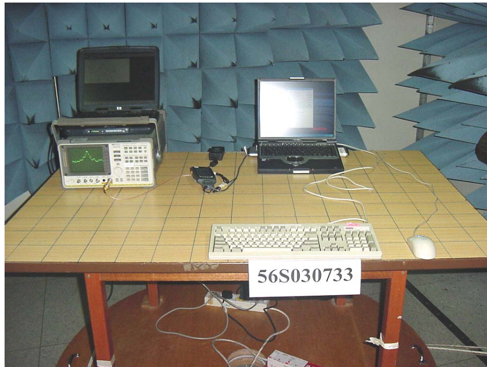
Spectrum Bandwidth Measurement Test Setup
