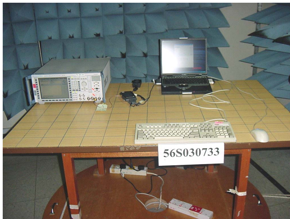
Maximum Peak Power Measurement Test Setup
