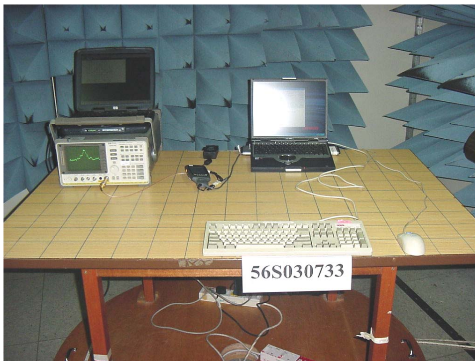
Peak Power Spectral Density Measurement Test Setup
