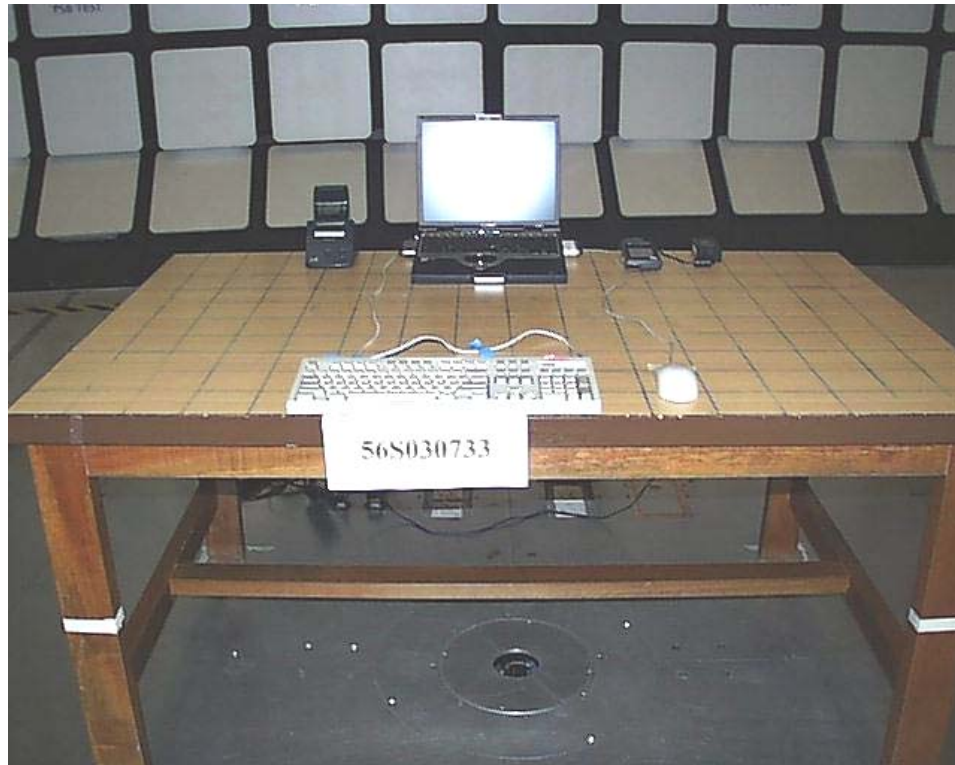
Radiated Emissions Setup (Front View)
