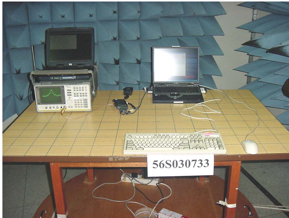
Number of Hopping Frequencies Measurement Test Setup
