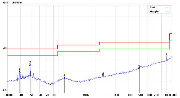
Site Polarization: Vertical Temperature: 25 Limit: FCC Part 15B Class B RE\_3 m Power: DC 3V Humidity: 55 %
