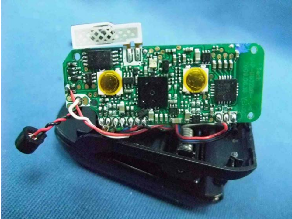
Bluetooth Headset Main PCB comp side
