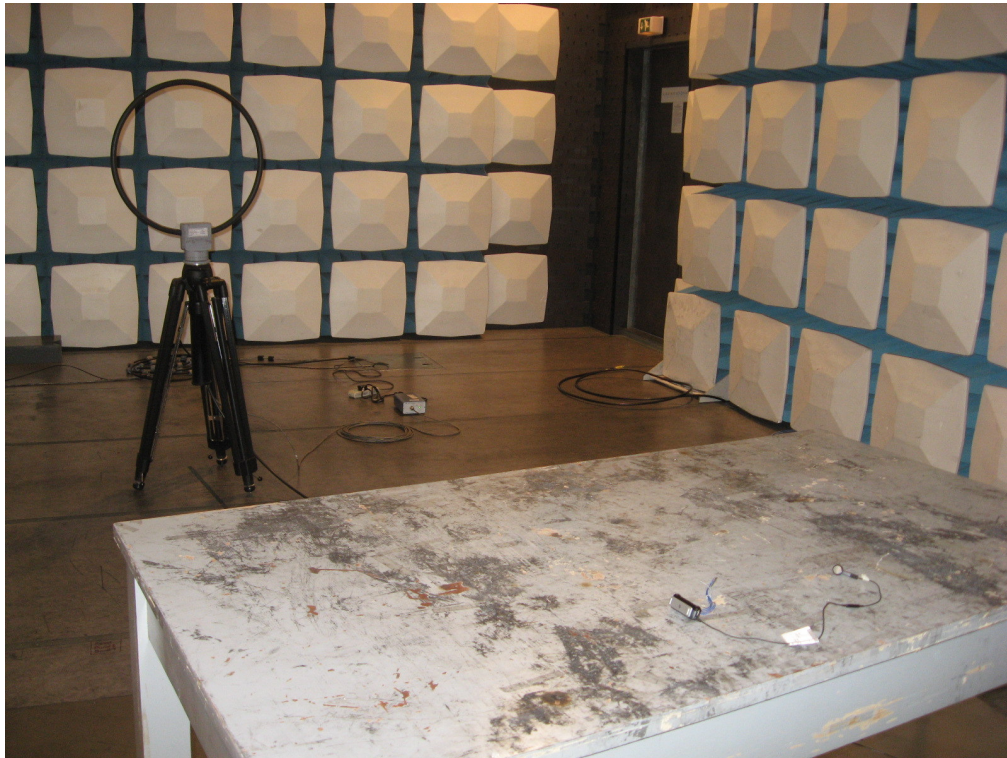
Set-up for Radiation Emission (Transceiver)
