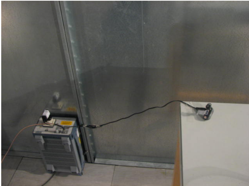
Set-up for AC wireline conducted emissions
