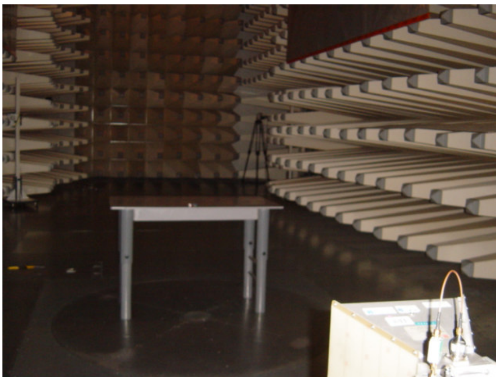
Set-up for Radiation Emission (Transceiver)
