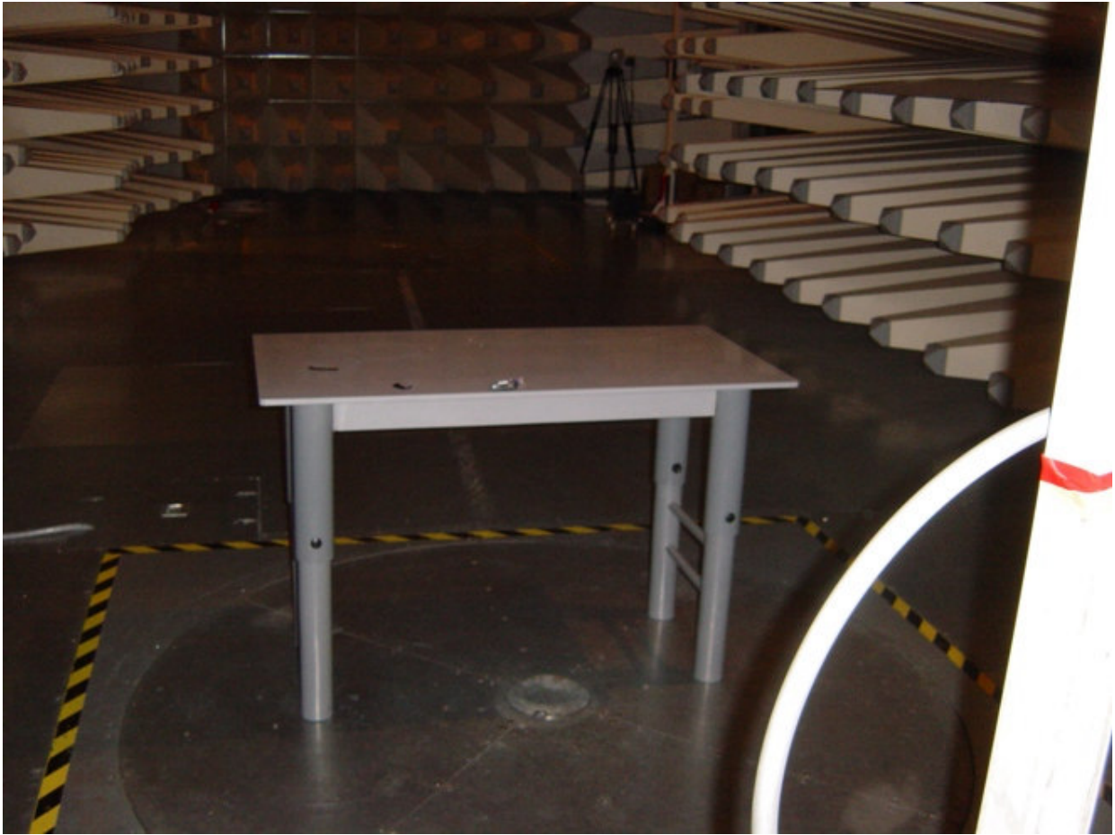
Set-up for Radiation Emission (Transceiver) – Loop Antenna
