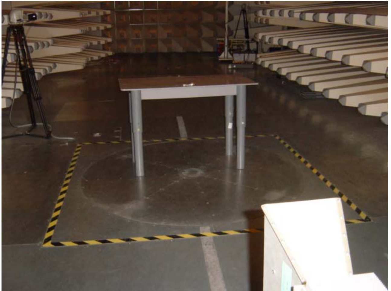
Set-up for Radiation Emission (Transceiver)
