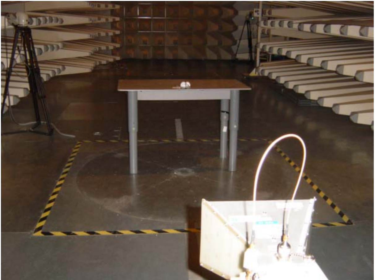
Set-up for Radiation Emission (Transceiver)
