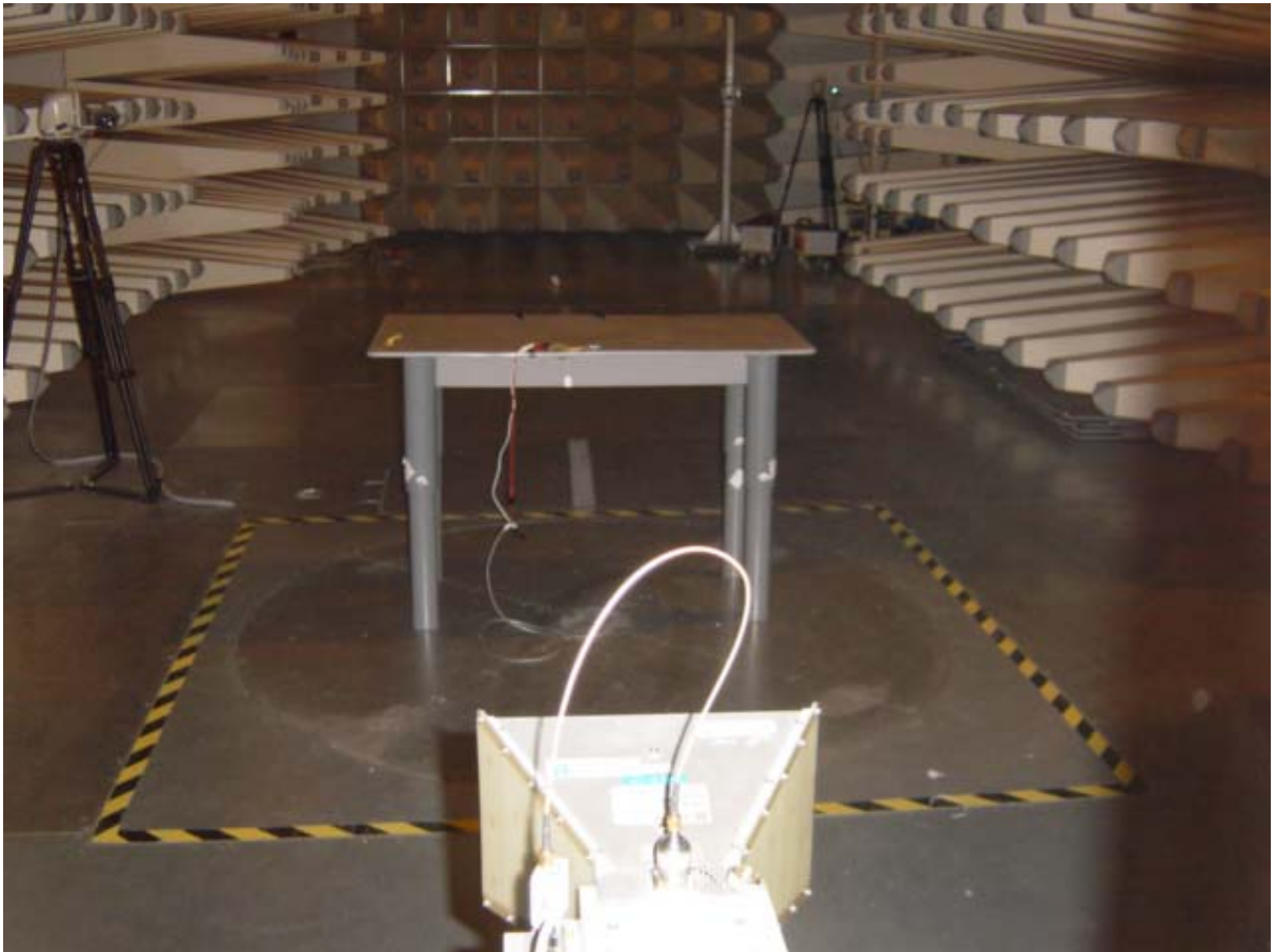
Set-up for Radiation Emission (Transceiver)
