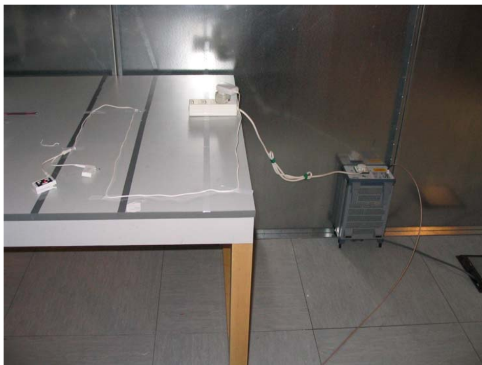
Set-up for Disturbance Voltage on AC mains
