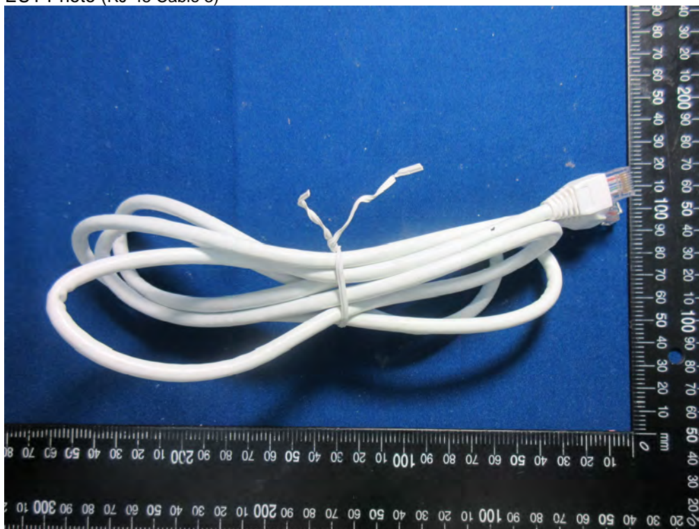
(13) EUT Photo (RJ-45 Cable 3)
