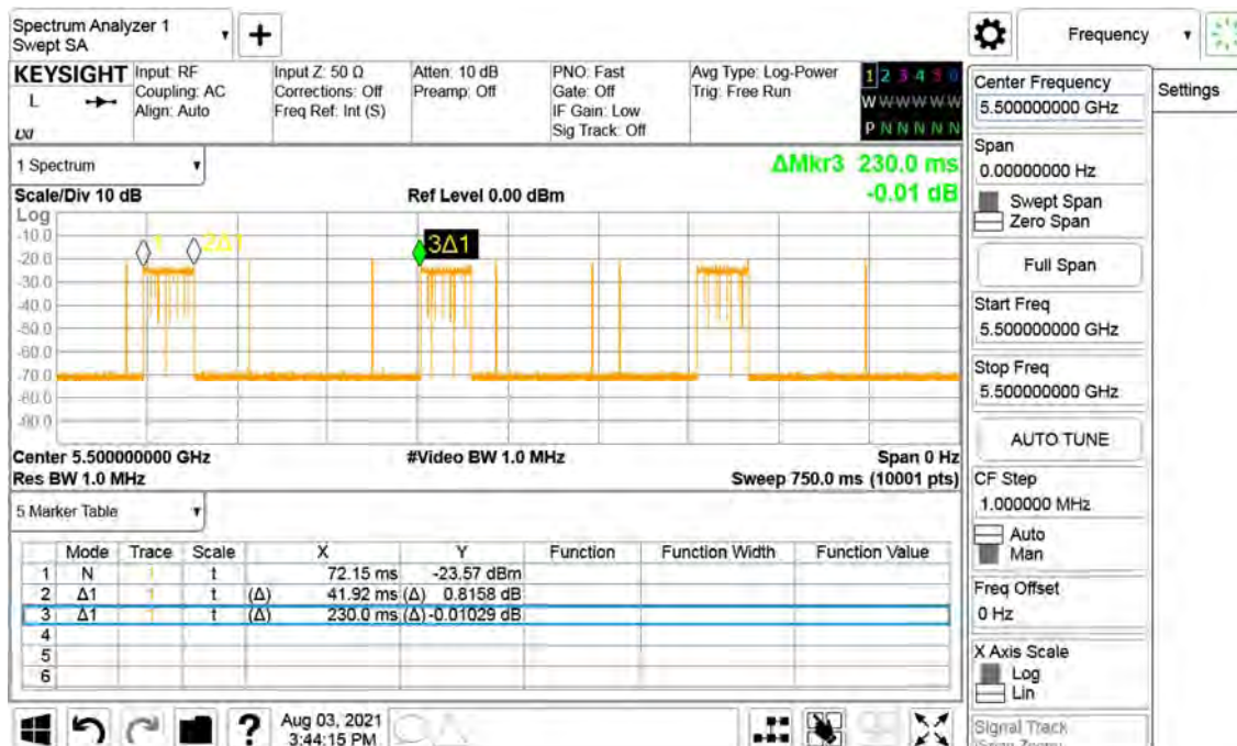
Plot of WLAN Traffic - 802.11ax (20MHz), 5500 MHz
