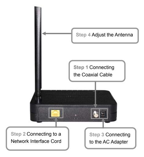
**Step 1:**Connect a cable by feeding the F-connector on the back of the cable modem. Ensure the center conductor of the 75 ohm coaxial cable is inserted directly into the center of the F-connector. Secure the coaxial cable by carefully threading the outer shell of the coaxial cable connector onto the F-connector in a clockwise direction until tight. Be careful not to over-tighten the connector or you may damage either the connector or the cable modem.
