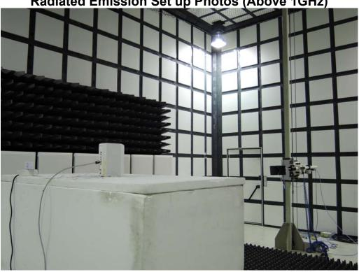
Radiated Emission Set up Photos (Above 1GHz)
