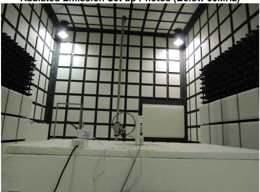
Radiated Emission Set up Photos (Below 1GHz)
