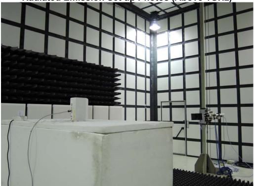
Radiated Emission Set up Photos (Front View)
