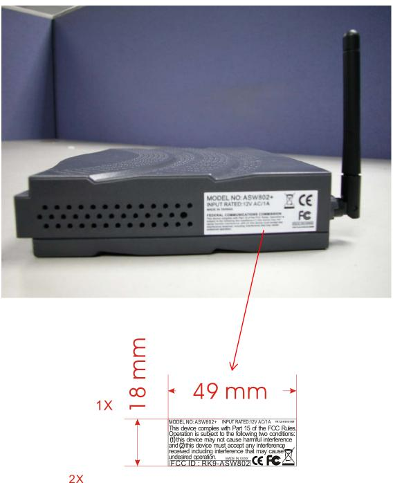
MODEL NO: ASW802+ INPUT RATED: 12V AC/1A PIN:7LB-01001G-100W This device complies with Part 15 of the FCC Rules. Operation is subject to the following two conditions: (1) this device may not cause harmful interference and (2) this device must accept any interference received including interference that may cause undesired operation.
